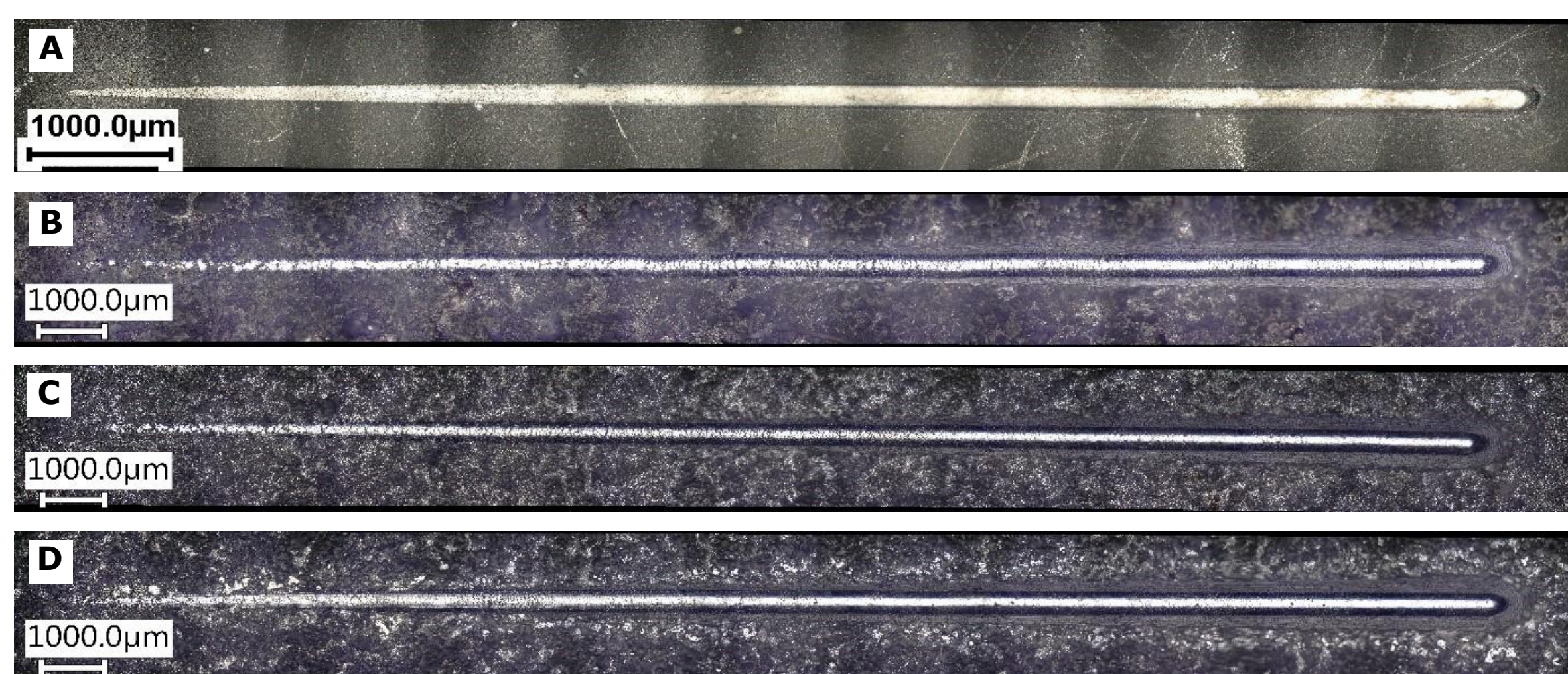
Fig. 2 Scratch test images of Ni-B and Ni-B/MoS 2 coating were A – Ni-B, B – Ni-B/MoS 2 (0.1), C – Ni-B/MoS 2 (0.3), D – Ni-B/MoS 2 (0.5)
